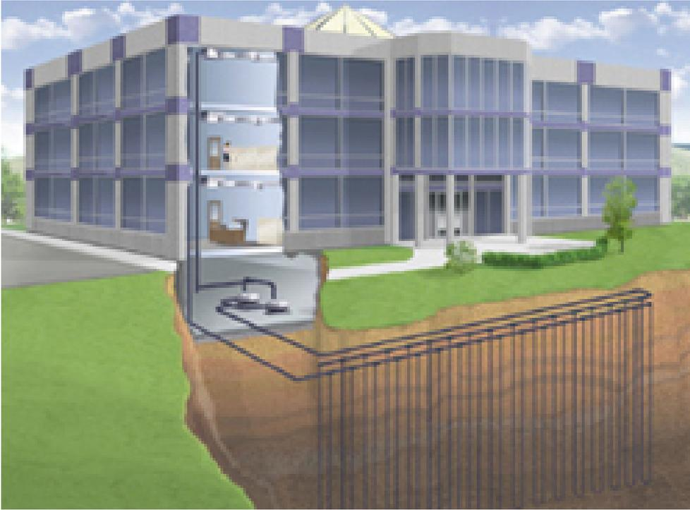
Vertical closed loop wells are used to provide ground source condenser water to heat recovery heat pump chiller plant, which is used to provide hot water heating and chilled water cooling
